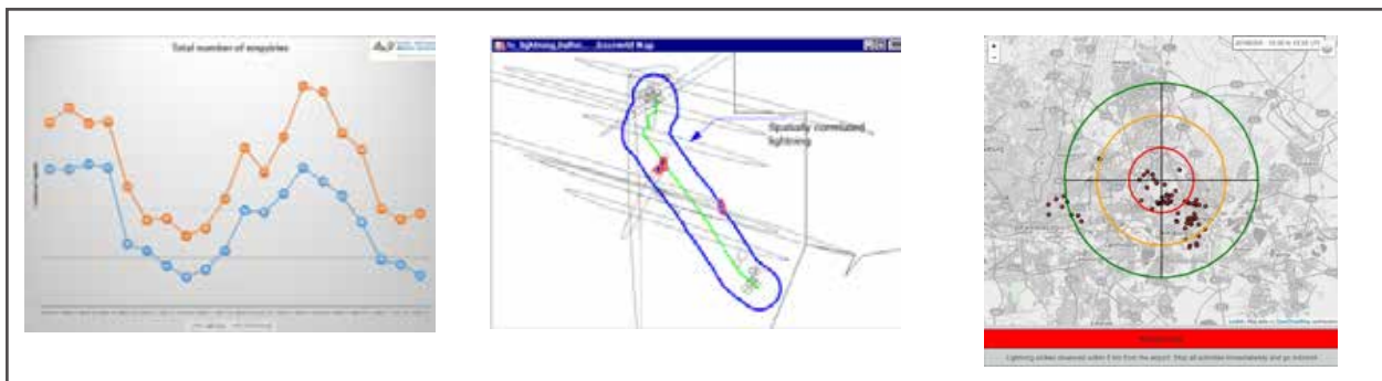
Figure 6: The typical amount of lightning (blue line) and total number (orange line) of queries received from the insurance sector (left), example of correlated lightning to power lines (centre) and a lightning alert system over O.R. Tambo International airport (right).
